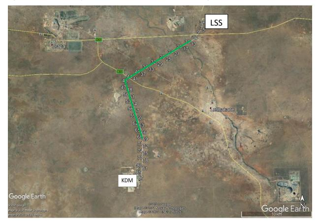
Figure 4: Location of the planned 132kV transmission line connecting KDM with Letlhakane Substation
